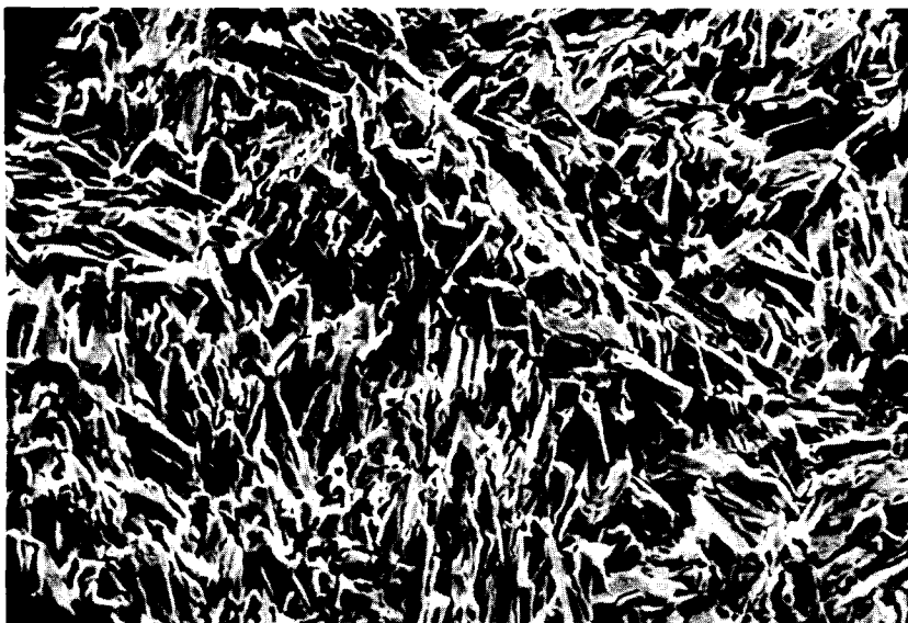
Fig. 10. Fully decomposed UHP, \times 400 .
