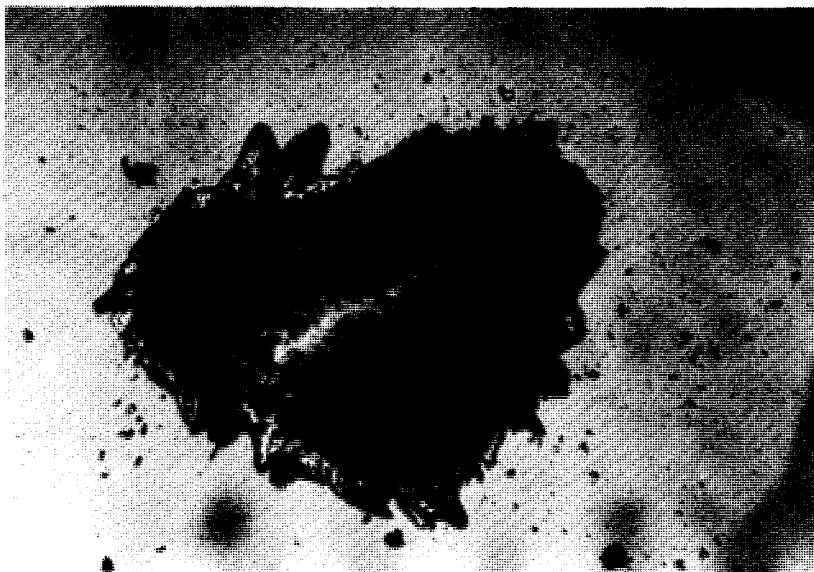
Fig. 12. 'Melted' UHP showing large crystals of urea, \times 120 .
